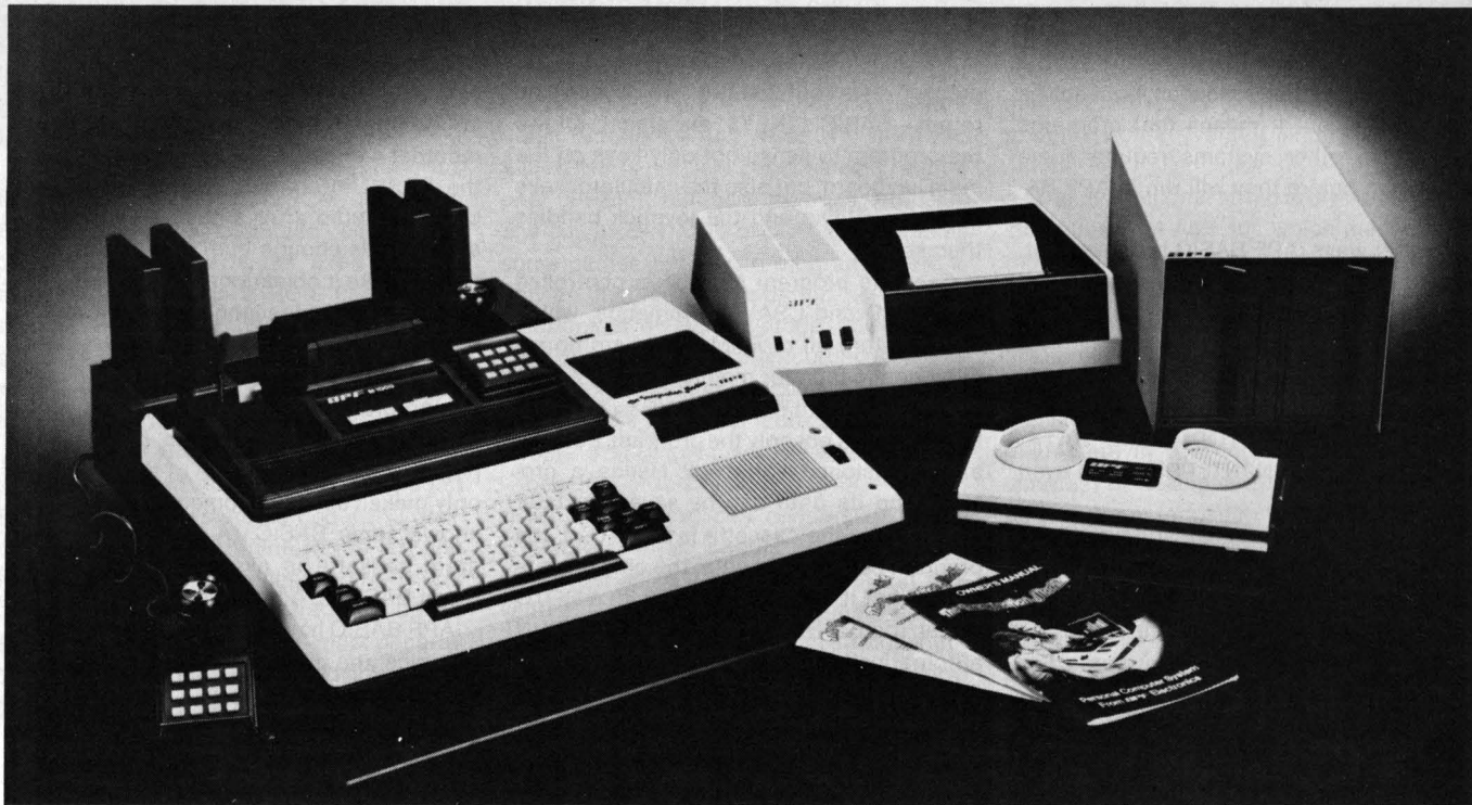
APF's Imagination Machine features a typewriter keyboard, two game-style controllers, a built-in cassette deck, a built-in microphone jack, a cartridge connector plus the expansion box to add on a printer, telephone modem, minifloppy disk or additional memory.
